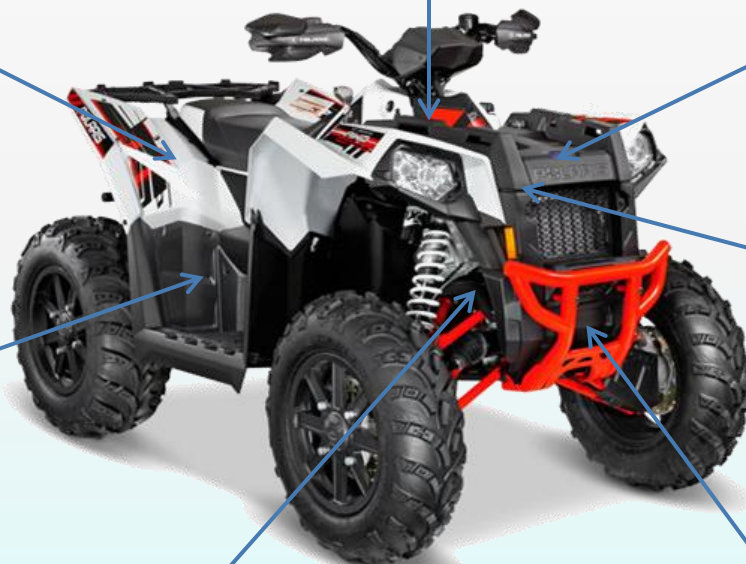
WELD-SKID, FRONT, BOLTED
