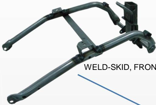
WELD-SKID, FRONT, BOLTED
